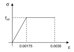
Modulus of elasticity of concrete is automatically calculated and displayed by the program using f<sub>ck</sub>, and the relationship (2.1-15)<sup>2</sup> of the code given below. User is given the option to override the code value and specify a user defined substitute.
